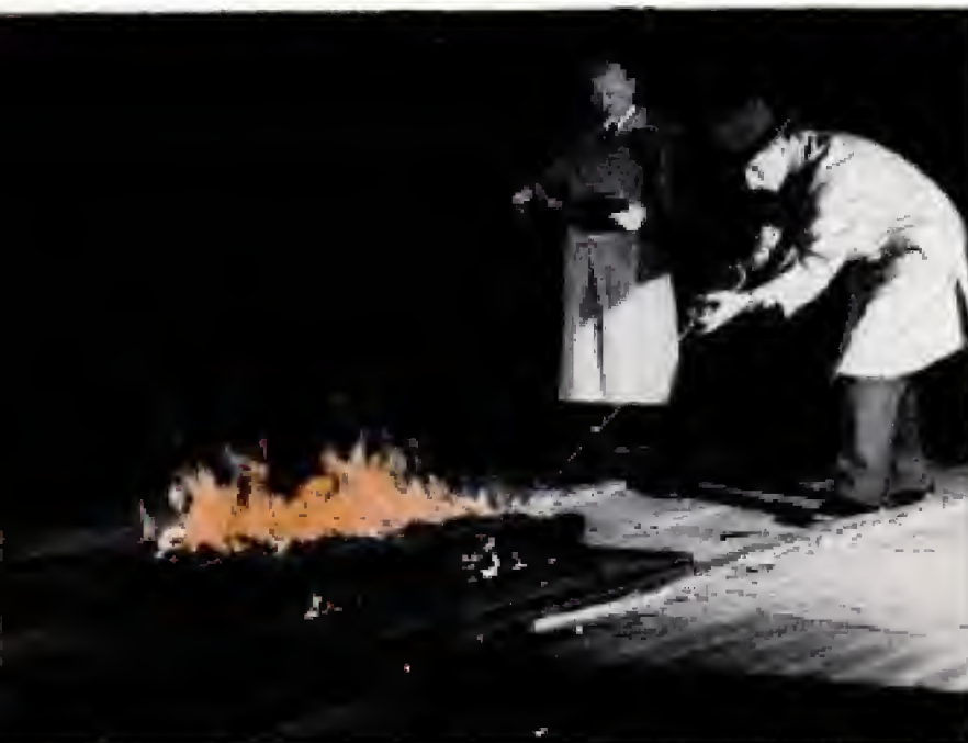
Engineers use a one-quart vaporizing-liquid extinguisher to put out blaze in cotton waste soaked with gasoline. Below, testing a carbon-dioxide extinguisher on a fire made by igniting two gallons of gasoline in a four-foot iron container
